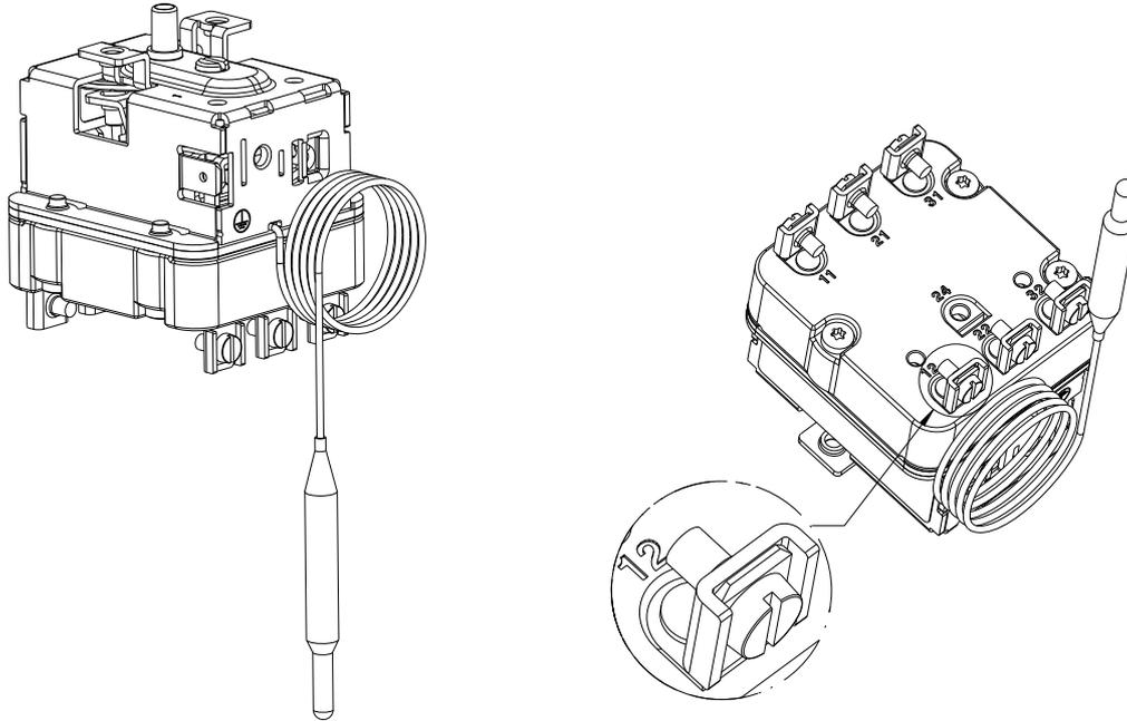
Electrical connection: screw connection up to 2.5 mm<sup>2</sup>
