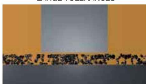
CONTAMINATION IN PRESENCE OF LARGE TOLERANCES
