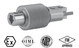
The low profile, high accuracy and sealing makes this load cell highly suitable for applications such as low profile platforms, weighing and packing machines, conversion of mechanical scales and variety of other applications where sealed cells are required. For hazardous environments this load cell is available with EEx ia IIC T6 level of approval as an option.
