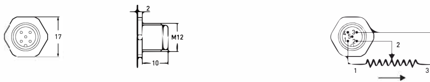
CN5A: 5 pin, M12 connector (optional - mating connector not included)
